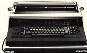
Hermit 21, an interface for the Hermes Toptronic 21 electronic typewriter, converts the Toptronic 21 into a full KSR printer-terminal. It features a 2,000 character print buffer and a 'white space skip' which increases print speed to 45 cps. It also has three modes of operation. Hermit 21, £402.50, is available from Duplex Communications at Dunton Bassett, Leicestershire, (0455) 209131.
